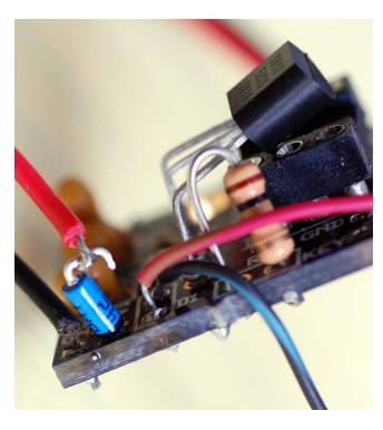
Install the BAT42 as shown in series with the positive lead from the battery. Note the banded end is connected to the board and the anode is connected to the battery. The LED was remoted via the red and black-blue wires.
