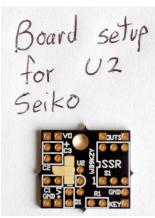
Boards will now have tape applied to mask off the holes for the "wrong" regulator.
